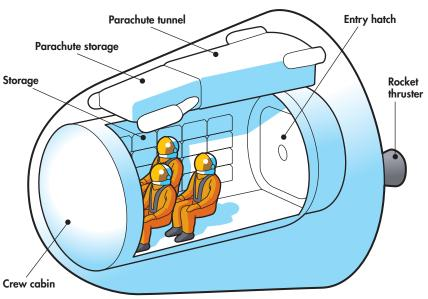
CAPSULE The crew transfer vehicle (CXV) capsule accommodates three or four crew members and their supplies. Its design is based on the Corona reentry vehicle used to return film from spy satellites—its blunt shape dissipates heat well and automatically orients the craft for re-entry. During the CXV's descent, two layers of inexpensive silicone and ceramic tiles protect it from thermal buildup, and the seats swivel to face the rear, easing G-force strain on the crew.
