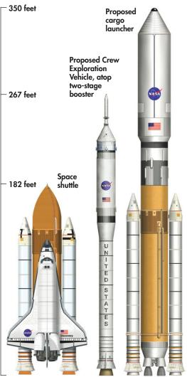
WORKING PLAN NASA's Crew Exploration Vehicle, or CEV, will send four astronauts to the moon by 2020, but a three-seat variant will also service the International Space Station by 2011. Although plans have yet to be finalized—these illustrations are from a proposal by space-systems contractor ATK a wingless space capsule will lift off atop a version of the space shuttle's solid rocket booster and a to-bedeveloped second-stage booster.
