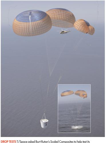
launch strategy. Scaled's Proteus aircraft dropped a guarter-scale mockup of the booster and capsule [left, in time-lapse image], which oriented itself flawlessly. A helicopter drop of the landing configuration [above] was also successful, although one chute failed to open completely.
